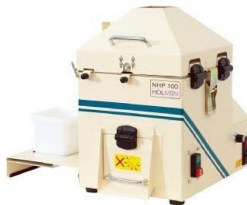
Figure 1. Holmen NHP 100 pellet durability tester
